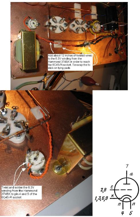
Figure 23. Wiring the 6.3V winding to the 6C45-Pi socket.
