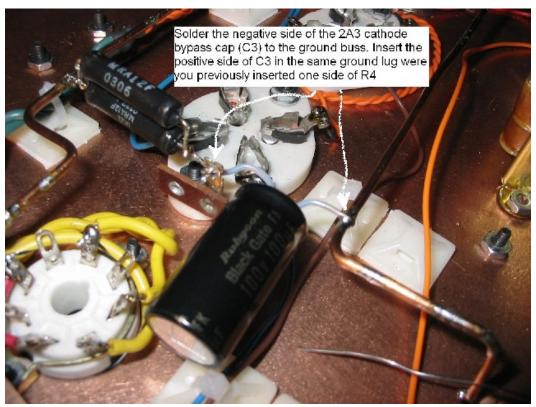
Figure 36. Installing C<sub>3</sub>.
