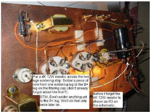
Figure 26. Wiring R<sub>3</sub> (part 1).
