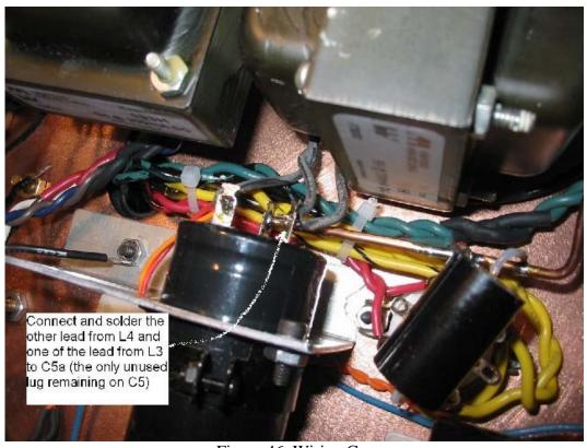
Figure 46. Wiring C<sub>5a</sub>.
