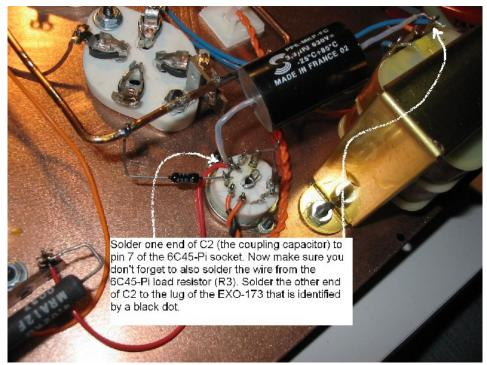
Figure 33. Wiring the coupling capacitor  $(C_2)$ .
