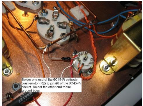
Figure 31. Wiring R<sub>2</sub>.
