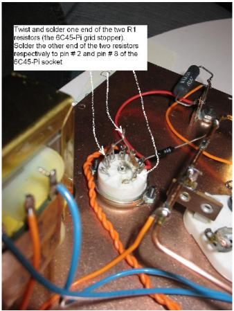
Figure 32. Wiring the grid stopper resistors  $(R_1)$ .
