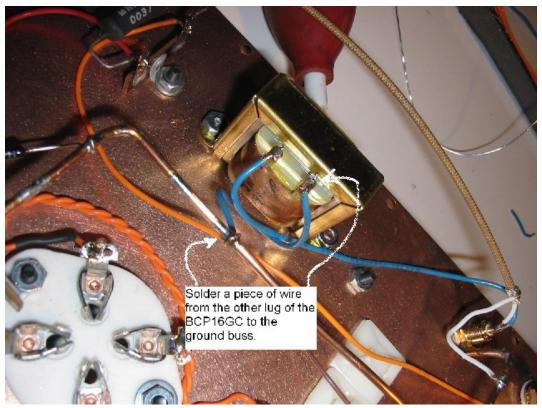
Figure 41. Final wiring of L<sub>1</sub>.
