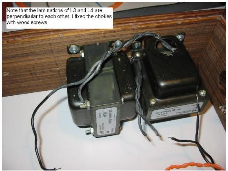
Figure 5 Close up of the PSU chokes (L3 and 14 on the schematic of the amp)
