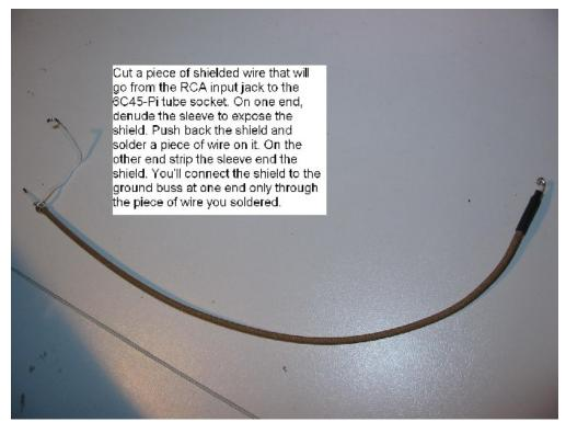
Figure 38. Preparing the input cable
