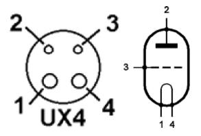
Figure 17. Pin out of the 2A3.
