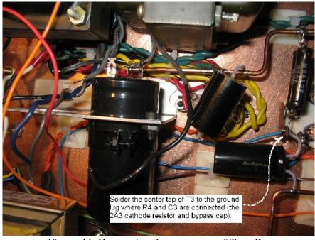
Figure 44. Connecting the center tap of T<sub>3</sub> to R<sub>4</sub>.
