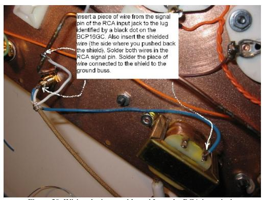
Figure 39. Wiring the input cable and  $L_1$  to the RCA input jack.
