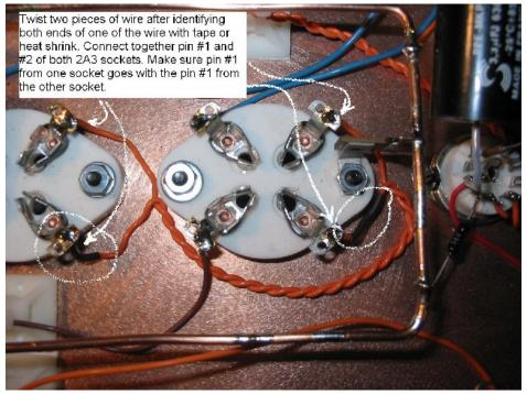
Figure 34. Wiring the heaters between the 2A3 sockets.
