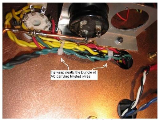
Figure 25. Tie-wrapping the AC wires bundle.
