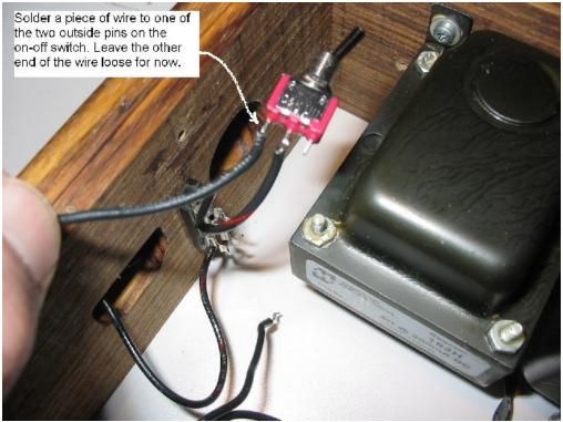
Figure 8. Wiring the on-off switch.
