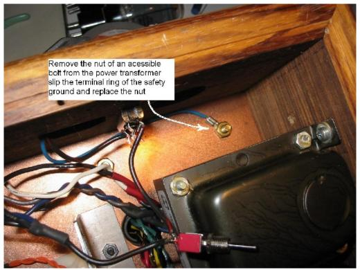
Figure 50. Wiring the safety ground (part 1).
