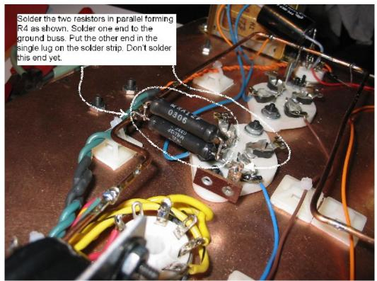
Figure 35. Installing R<sub>4</sub>.
