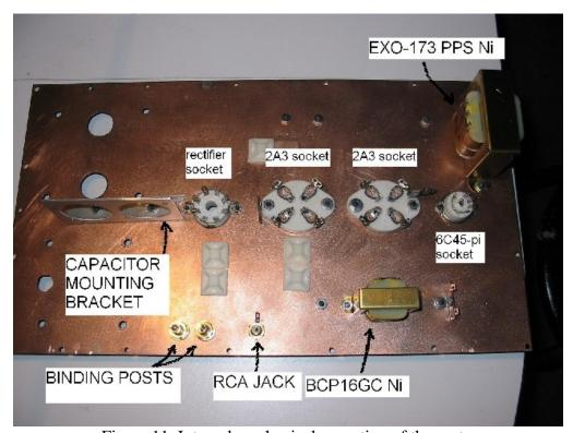
Figure 11. Internal mechanical mounting of the parts.
