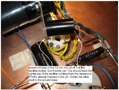
Figure 37. Wiring C<sub>4</sub>.
