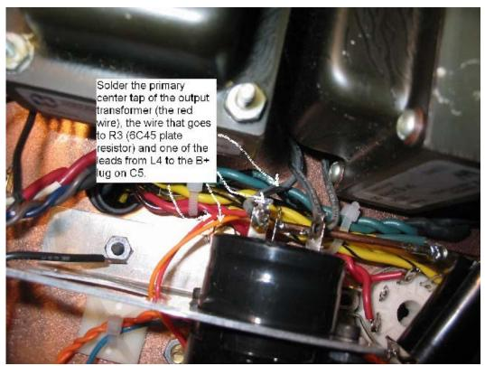
Figure 45. Wiring the  $B+(C_{5b})$ .
