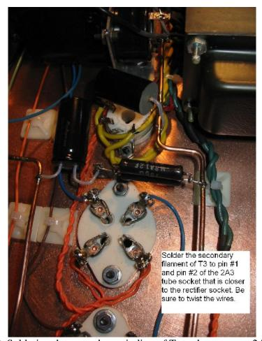
Figure 43. Soldering the secondary winding of T<sub>3</sub> to the rearmost 2A3 socket.
