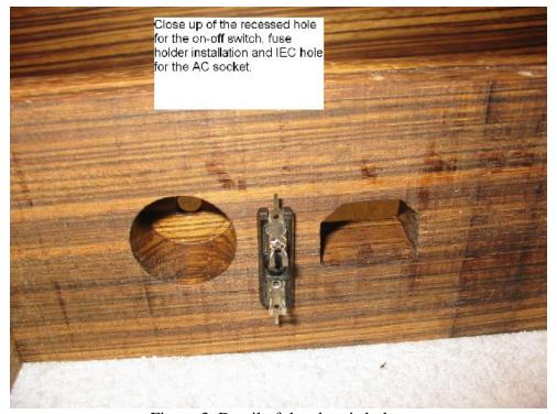
Figure 3. Detail of the chassis holes.
