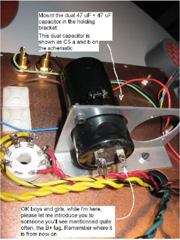
Figure 18. Installing  $\overline{C_5}$ .
